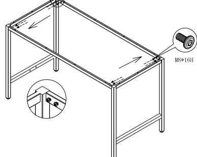
Please do not tighten the screws when assembling the top crossbeam.
