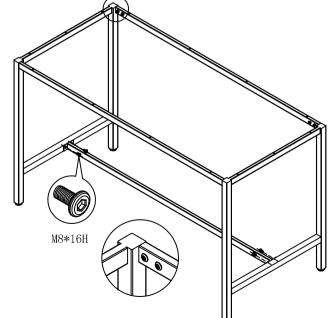
Please tighten the screws after Assembled all the beams.
