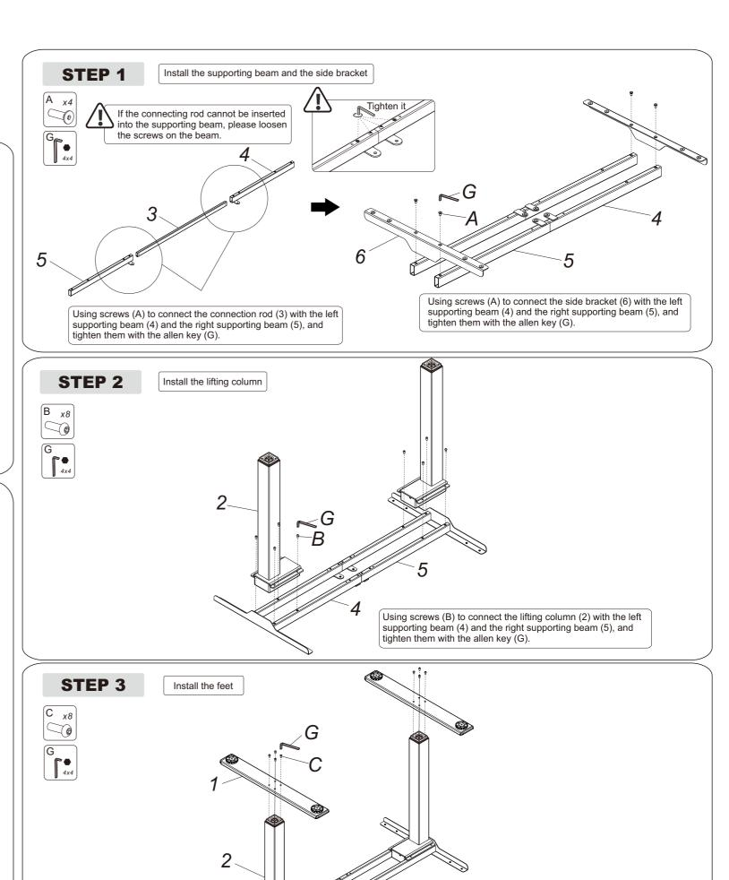
Connect the feet(1) and the lifting column (2) with screws (C),
