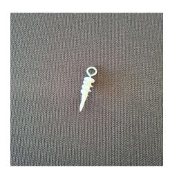
Step 1- prepare the metal eyes Screw in the metal eyelet into the plaster mate plugs
