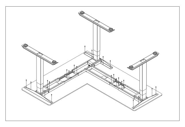
Mount the control box to the frame, fix the handset with 2pcs screws ST4x20. Connect the cables and zipped it with cable tie.
