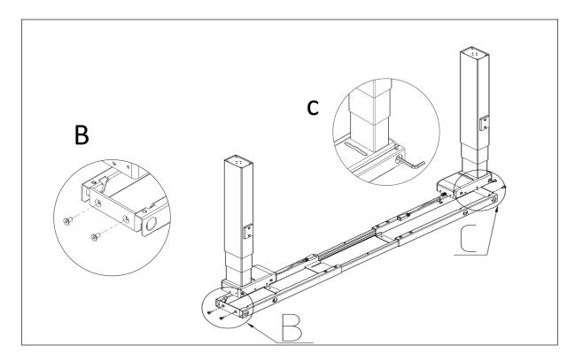
Install the two table feet with Screws 8 pcs M6x16,
