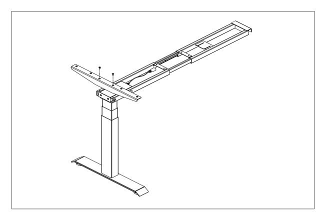
Connect the return frame to the single workstation and fixed with 2 hand bolts. Fix the centre brackets with 2pcs screws M6x10.
