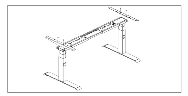
Mount the tabletop and fix it with 14 pcs screws ST4x20; Tighten the screws like D display to fix the top frame.Fix the centre bracket with 2 pcs screws M6x10
