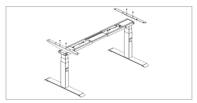
**Step 5**Mount the tabletop and fix it with 14 pcs screws ST4x20; Tighten the screws like D display to fix the top frame. Fix the centre bracket with 2 pcs screws M6x10
