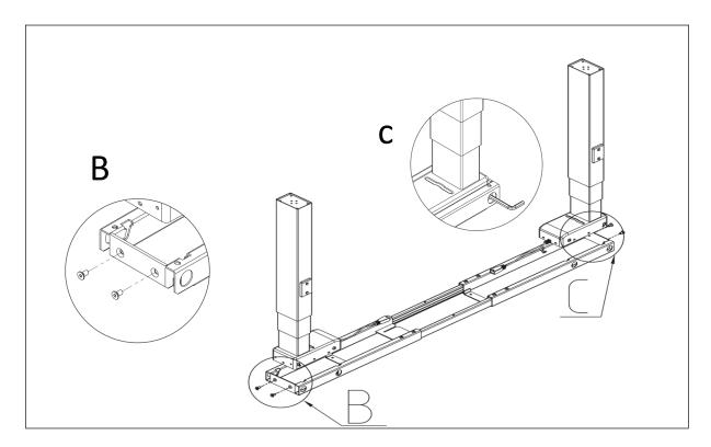
**Step 3**Install the two table feet with Screws 8 pcs M6x16, Install the 4 pcs leveling pads
