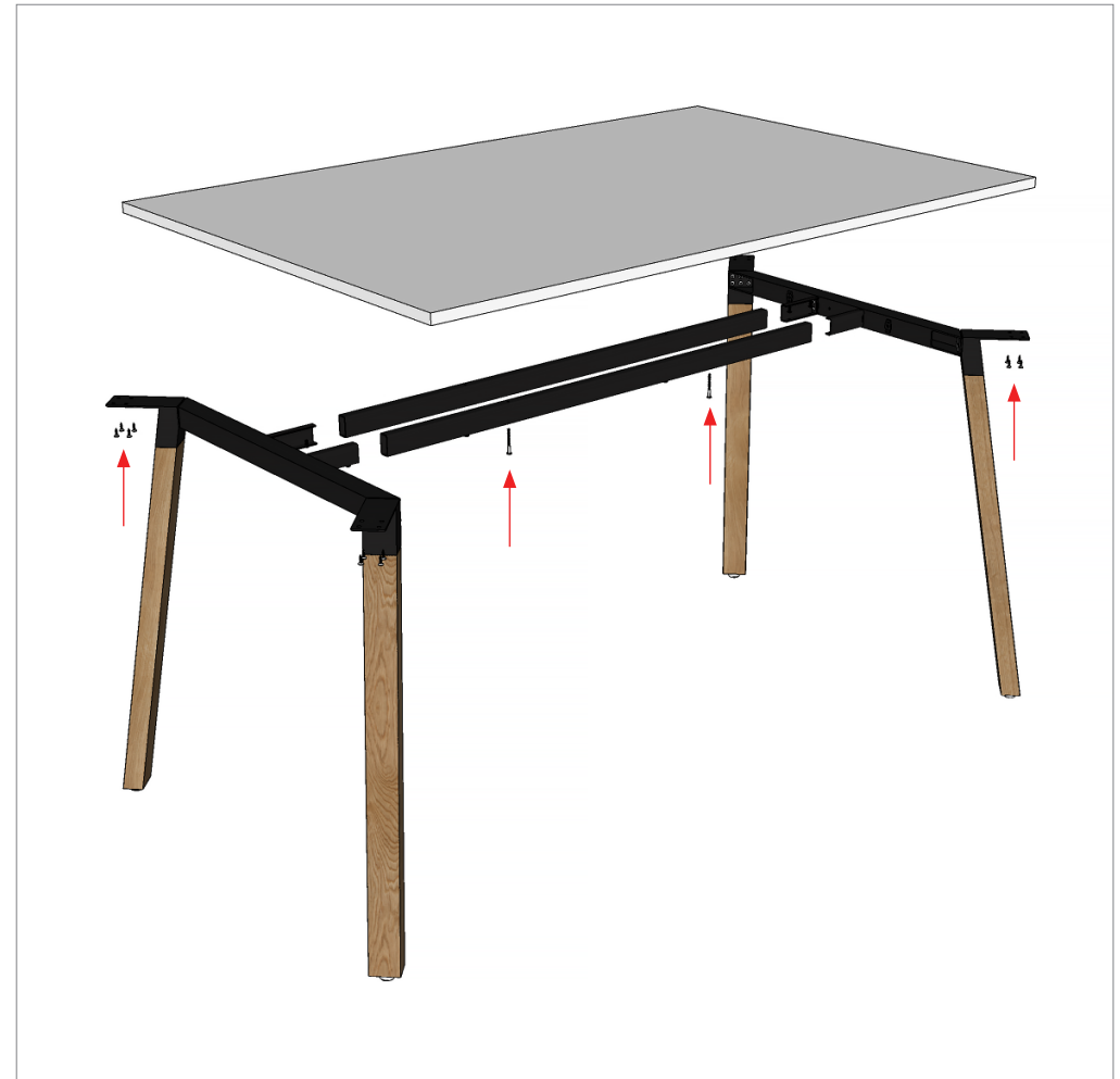
STEP 4: Attach worktop to frame.
