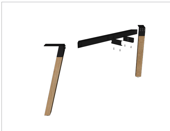
STEP 1: Assemble 2x end leg frames to the legs. Total 6 x M12 per leg.
