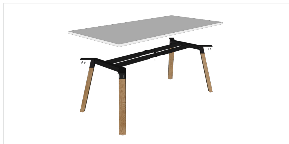
STEP 4: Fix worktop to frame using 4 x 23mm screw per leg, 1 x 23mm screw per rail.
