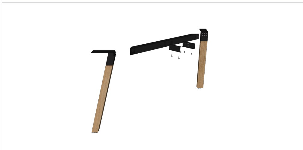
STEP 1: Assemble 2x end leg frames to the legs. Total 6 x M12 per leg.
