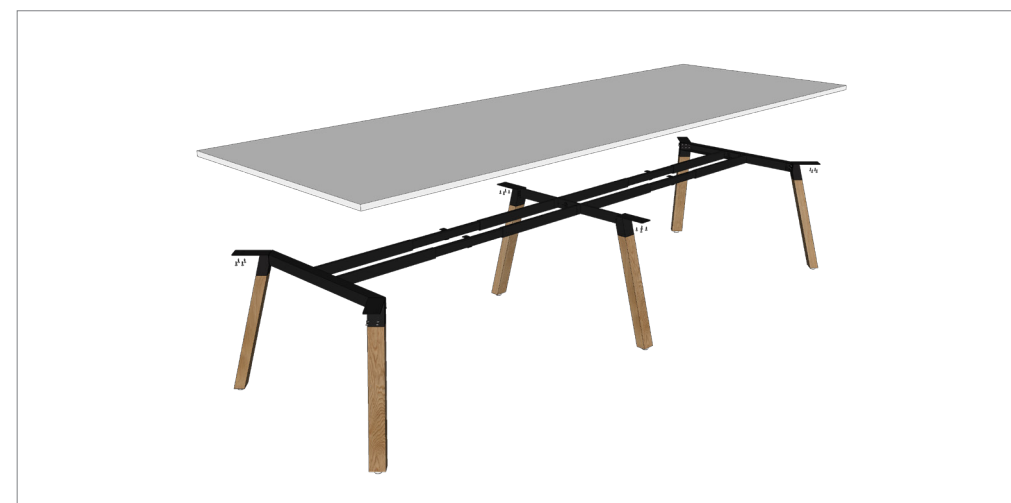
STEP 5: Fix worktop to frame using 4 x 23mm screw per leg, 1 x 23mm screw per rail.
