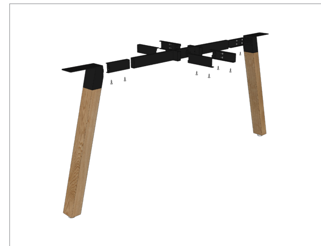
STEP 3: Assemble the mid leg using bolts provided in the spreader bar kit. Mount the rail to the centre mounting point.
