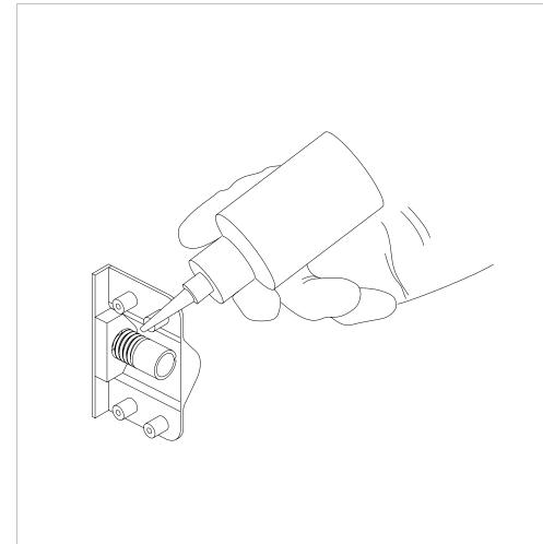
**STEP 14:** Once the desired locking setup is achieved, remove the latch from the door. Mark the correct position of the threaded tube and unscrew. Apply LOCTITE or similar product on the thread so it doesn't loosen over time. Adjust the threaded tube back to the original position.
