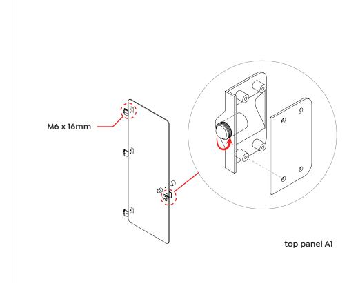
**STEP 11:** Bolt the hinges, handle and door lock to the glass door. The threaded tube on the door latch allows adjustment for a tigther closing. Might requiere a few trials to find the perfect position.
