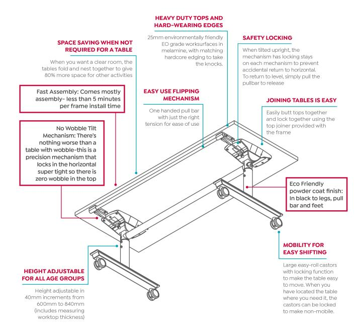
$Standard\ Worktop\ Sizes:\ Frames\ to\ suit\ top\ lengths\ of\ 800-2100mm,\ and\ top\ widths\ of\ 600-750mm$
