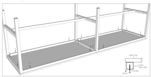
**COMPLETE:** Pre-drill holes into the worktop, place worktop on a clean, flat surface and fully tighten the worktop to each rail using the provided screws. Using 2 people rotate table into upright position.
