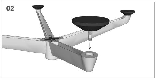
Screw the 4 glides into the base of the large feet, leaving the glides one turn from tight (then they can be adjusted easily if the floor is uneven).
