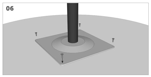
Fully tighten the last 4 self tapping screws into the work surface.
