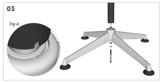
Place the feet tube into the cross collar, making sure the notch in the bottom of the tube is in-line with the bump inside the cross collar  $Fig\ A$ . Fully tighten the large M10 bolt, spring washer and flat washer through the gasket and collar into the tube.
