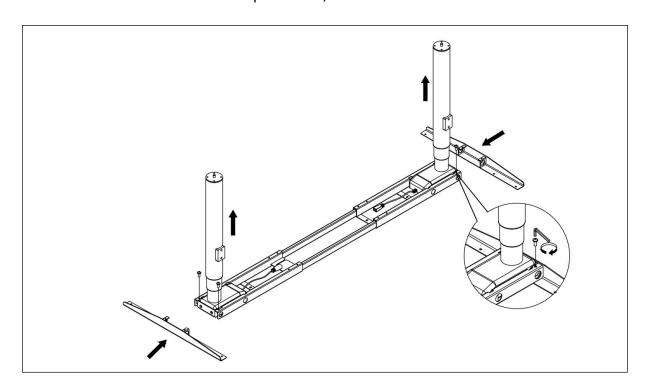
**Step 4** Install the leveling pads
