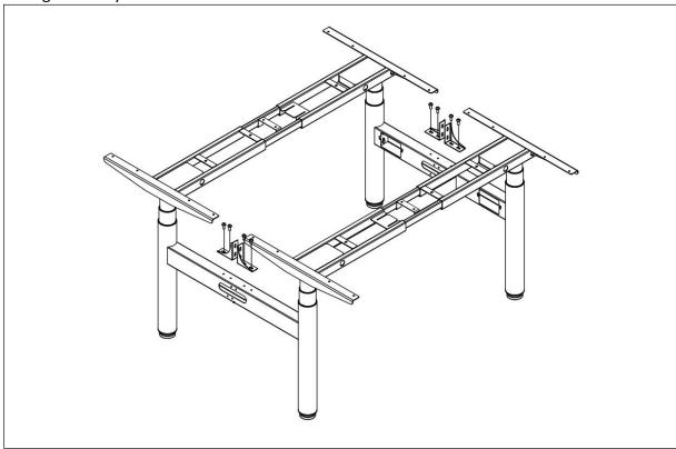
**Step 7**Fix the table top with 30 pcs screws ST4x20 ,Fix the handset with 4 pcs screws with ST4x20 Install the centre bracket with 2 pcs screws M6x10
