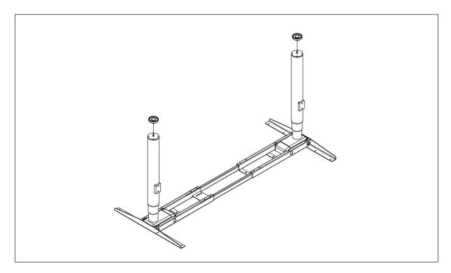
**Step 5**Install the connected pipe with 8 pcs screws M8x10
