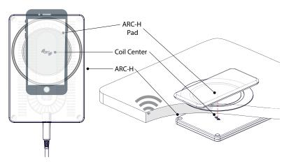
The ARC logo identifies the coil center which must be aligned with the resonator pad
