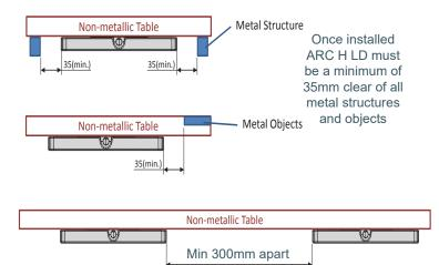
Every ARC H LD must be installed a minimum of 300mm apart
