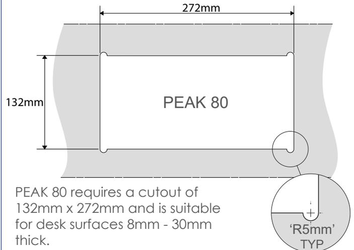
PEAK 80 requires a cutout of 132mm x 272mm and is suitable for desk surfaces 8mm - 30mm thick.
