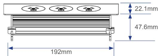
\*Corners of cut-outs must not be radiused. Suitable for table tops 10mm-30mm thick, and secured by the supplied 4x screw clamps.
