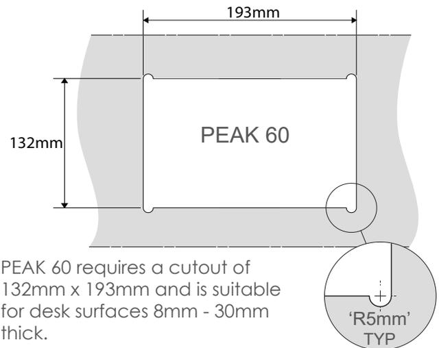
PEAK 60 requires a cutout of 132mm x 193mm and is suitable for desk surfaces 8mm - 30mm thick.
