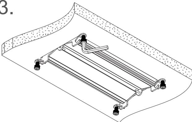
Screw the provided M8 x 20mm cap head fixing bolts through the fixing mounts until the unit is secure. Ensure that your cables are suitably managed - Solutions are available from OE Elsafe Australia.
