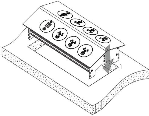
Place PEAK into the cutout ensuring that any cables are not trapped in the process.
