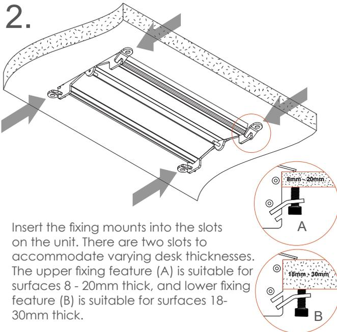
Insert the fixing mounts into the slots on the unit. There are two slots to accommodate varying desk thicknesses. The upper fixing feature (A) is suitable for surfaces 8 - 20mm thick, and lower fixing feature (B) is suitable for surfaces 18-30mm thick.
