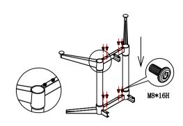
Slide Both The Bottom And Top Cross Bar Into The Left &Right Hand Side End Uprights - Attach Cross Bars WithM8 Bolts ( Do Not Completely Tighten Bolts )
