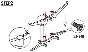
Slide Both The Bottom And Top Cross Bar Into The Central Uprights - Attach Cross Bars With M8 Bolts ( Do Not Completely Tighten Bolts )
