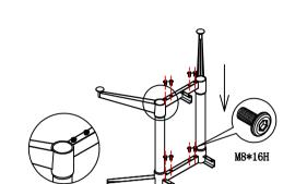
Slide Both The Bottom And Top Cross Bar Into The Left &Right Hand Side End Uprights - Attach Cross Bars WithM8 Bolts ( Do Not Completely Tighten Bolts )
